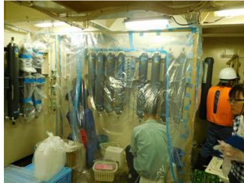
Clean technique and filtration using a polycarbonate filter (pore size is 0.2 \mu\text{m} )
